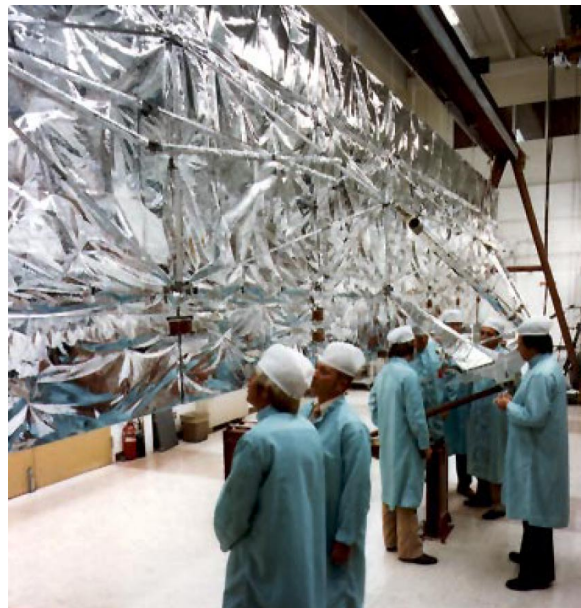
Figure G-12. SeaSat antenna and structure in deployed state with thermal blanketing.
