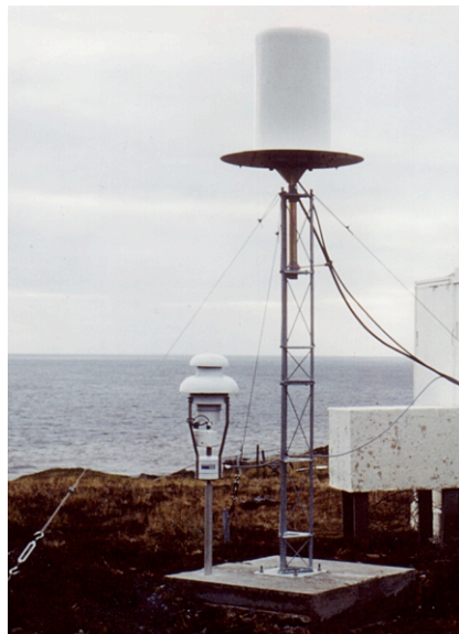
Figure 6: 2 m tower on a concrete block (Marion Island/MARA)
