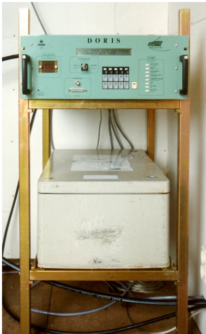
Figure 3: DORIS beacon 1.0 (top) and Battery case (bottom) in a homemade rack
