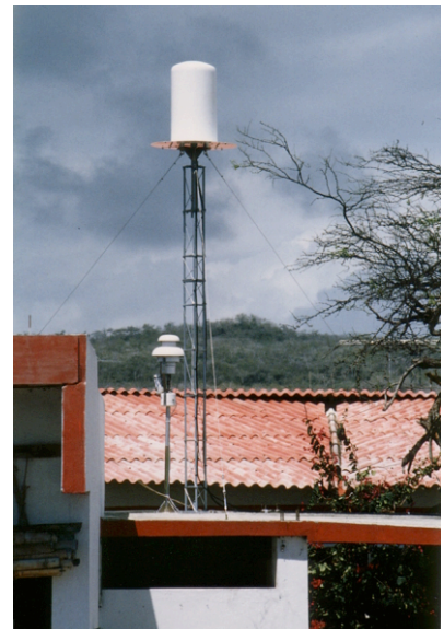
Figure 7: 3 m tower on the upper terrace of a building (Galapagos/GALA)
