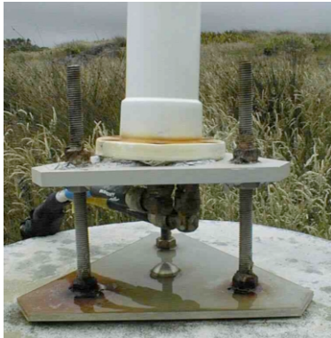
Figure 17 Antenna tilt resulting from the corrosion of the base plate (Amsterdam/AMSB)
