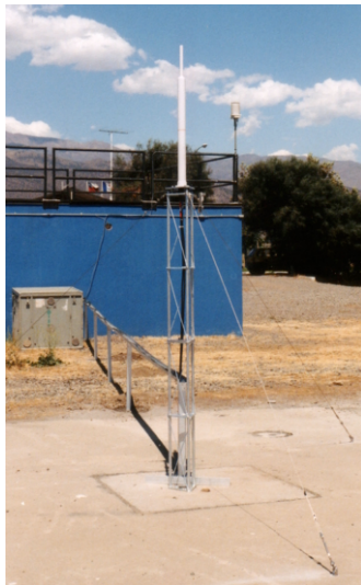
Figure 13 Standard layout: 2 metre tower, guyed (Santiago/SAOB)
