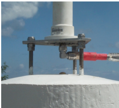
Figure 19 Base plate embedded in a pillar. (Nouméa/NOWB)
