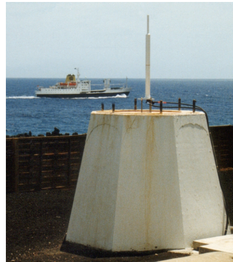
Figure 15 The first DORIS antenna mounted on a concrete pillar (a former antenna pedestal) (Ascension/ASDB)
